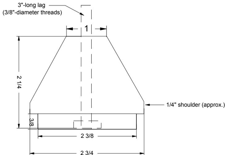
The bolt is threaded through a hole bored the length of of the jig, the head recessed flush with the back edge. The spigot at the rear was sized to fit my chuck. To increase the grip on the stopper blank 3/8" hole, I wrap the exposed threads with non-waxed masking tape to act as a shim. Nothing fancy here!
